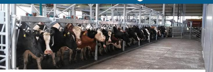
The Rapid Excellent is an advanced side-by-side Rapid Exit milking parlour, a proven concept for good and reliable milking. Characteristic is its solid, robust construction. The breast barriers move vertically upwards by means of an electro-hydraulic system and do not swing forward and therefore allows the cows to exit the milking parlour simultaneously via the broad exit lane.
