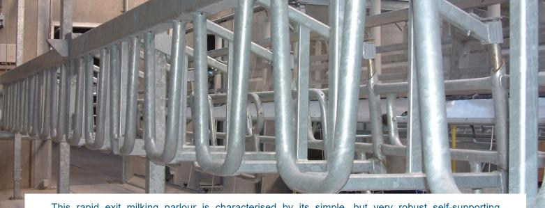
This rapid exit milking parlour is characterised by its simple, but very robust self-supporting construction. Due to its pneumatic controls, it is an economically attractive milking parlour. Despite its low overall height, this milking parlour has a more than sufficient passage height. Thanks to a modular construction system, it can be installed quickly in both new or renovated buildings.
